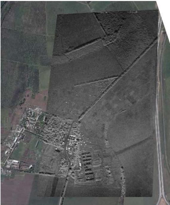
Fig. 3: SAR image (45 looks) formed by using the built-in geometric correction is imposed on the Google Map image.
