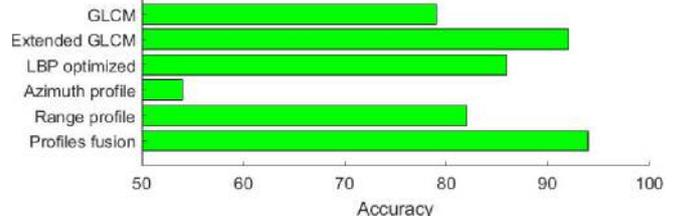
Figure 6. Recognition accuracy for different feature sets with SVM.
