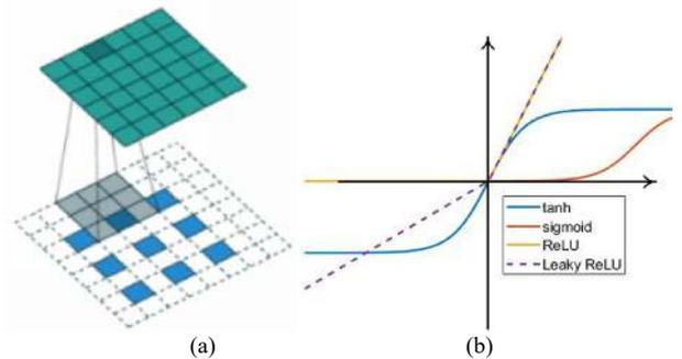
Figure 3. Typical CNN building blocks (a – convolution, b – activation functions)
